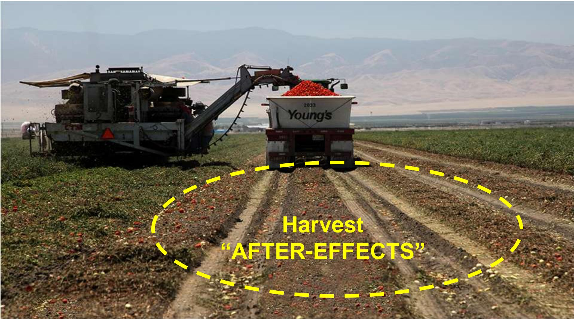
Vine trash PLUS bed erosion and soil compaction from repeated trips over tomato beds by tractors, harvesters and bin trailers weighing up to 20 tons centered over narrow wheels, leave after effects that need BIG ag tillage solutions for next year's crop to flourish.
