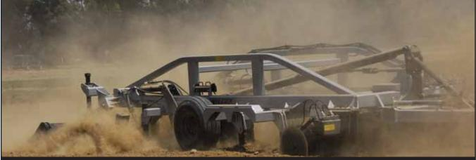
Agressive action from Rotor mulches organic matter back into the soil and leaves level surface for sizing and firming by Two Stage Roller..
