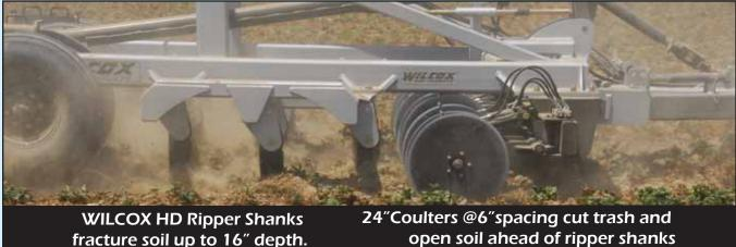
fracture soil up to 16" depth.
