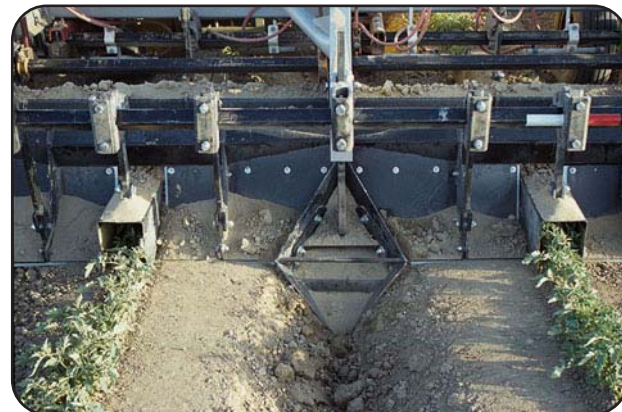
The Wilcox Performer is a simple, ground driven and extremely productive implement. Without the usually troublesome chain boxes, drive lines, gear boxes, and PTO components.
