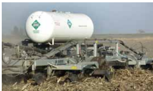
10,000 Lb. carrying capacity supports pre-herbicide & pre-fertilizer application.
