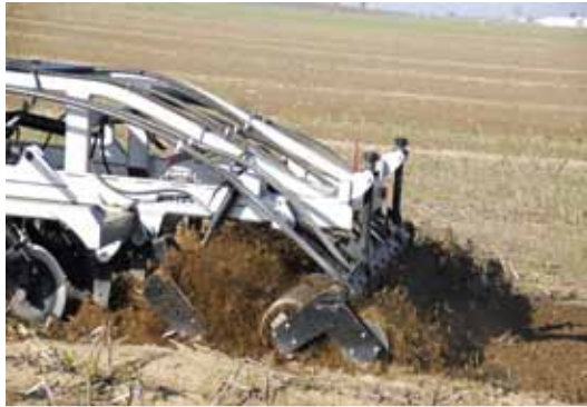
Double action rotors and two stage roller system at work.
